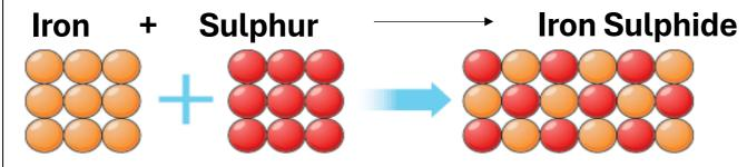
Properties of iron sulphide are different to the two elements – this reaction is irreversible.
